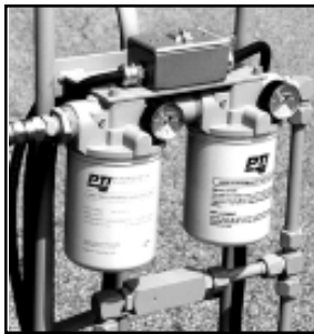
Pressure gauges let you know when a filter change is due.
