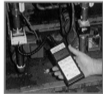
For flow measurement only clip flow sensor on RotoFlow™.
